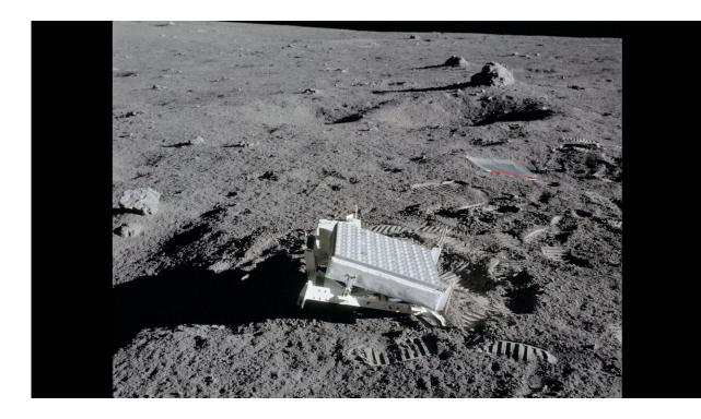
A close-up view, taken on Feb. 5, 1971, of the Laser Ranging Retro-Reflector (LR3), which the Apollo 14 astronauts deployed on the Moon during their lunar surface extravehicular activity. Credit: NASA
