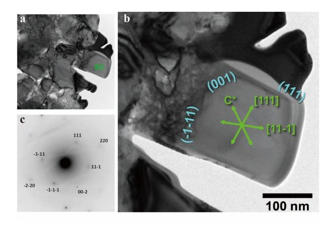
Since the crystals of microdiamond are finer than 1 micron, they were confirmed by the latest analytical techniques such as Raman spectroscopy, soft X-ray spectroscopy, and transmission electron microscopy. Credit: Professor Tadao Nishiyama
