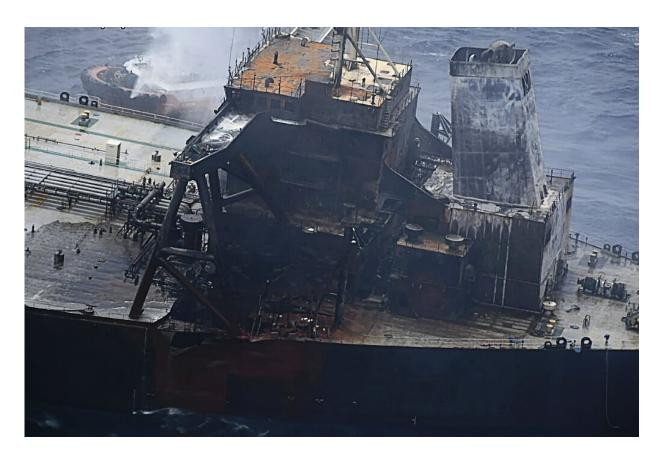
The fire started after an explosion in the boiler room while the New Diamond was on its way to the Indian port of Paradip
