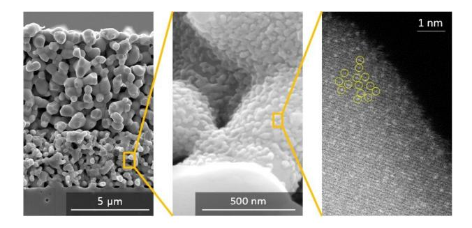
(left) solid oxide fuel cell electrode(center) a single atom catalyst formed on the surface inside the electrode.(right) platinum atom dispersed on the catalytic surface (bright point: platinum atom). Credit: Korea Institue of Science and Technology(KIST)
