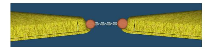
Illustration of Porath's experiment showing a DNA molecule, through which an electric current is flowing, that is bound by two nanoparticles (orange circles) to the electrodes (yellow). Credit: Hebrew University
