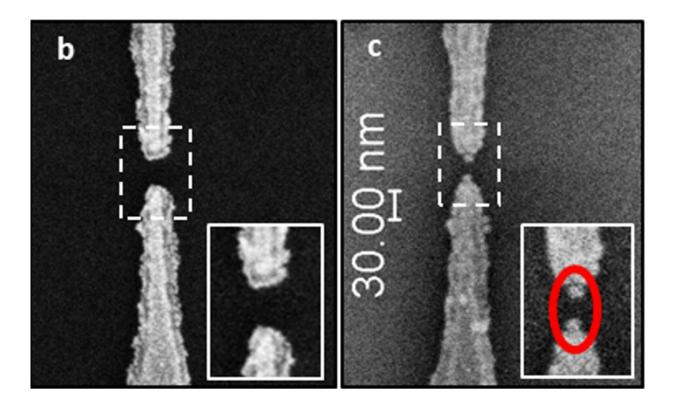
Image from an electron microscope showing electrodes with a single DNA molecule. Right image shows molecule (see the nanoparticles circled by a red ellipses), on the left without a molecule. Credit: Hebrew University of Jerusalem
