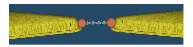
Illustration of Porath's experiment showing a DNA molecule, through which an electric current is flowing, that is bound by two nanoparticles (orange circles) to the electrodes (yellow). Credit: Hebrew University
