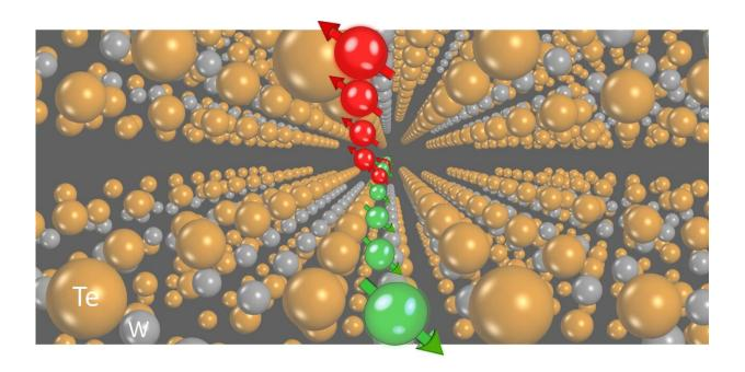
Fig 1. A schematic presentation of spin Hall effect in Weyl semimetal 1T' WTe2, showing the separation of spin-polarized electrons (up and down spin) on the surfaces of a sample by just passing a charge current. Credit: Bing Zhao
