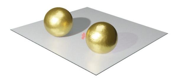
Shadow stealer. The absorption of light by a gold nanoparticle is reduced—and the shadow weakened—when a dye molecule (red) is placed nearby. With experimental improvements, the nanoparticle could become transparent. Credit: J. Zirkelbach/Max Planck Inst. for the Science of Light, via *Physics*, DOI: 10.1103/Physics.13.141
