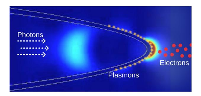
Light moves through a fiber and stimulates the metal electrons in nanotip into collective oscillations called surface plasmons, assisting electrons to leave the tip. This simple electron nano-gun can be made more versatile via different forms of material composition and structuring. Credit: Ali Passian/ORNL, U.S. Dept. of Energy
