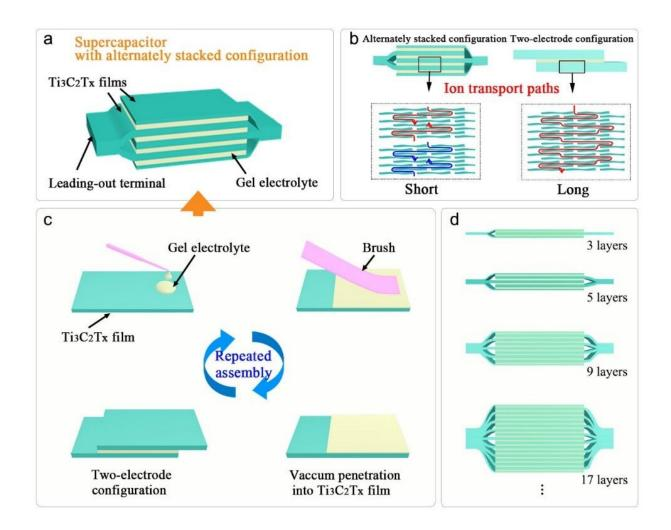
Assembly of the supercapacitor with an alternately stacked electrode configuration. Credit: PAN Qijuan
