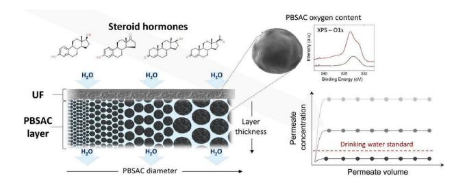
Filtration systems with the semipermeable membrane (Ultrafiltration – UF) and a layer of activated carbon (polymer-based spherical activated carbon – PBSAC). Credit: IAMT/KIT
