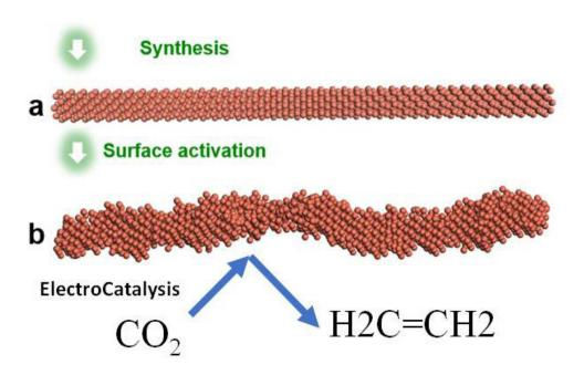
Illustration of the ElectroCatalysis system which synthesized the smooth nanowire and then activated it by applying a voltage to get the rough stepped surface that is highly selective for CO2 reduction to ethylene. Credit: Yu Huang and William A. Goddard III
