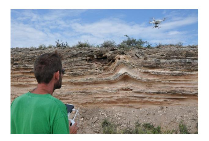
Southwest Research Institute uses drone-based, remote-sensing techniques to digitally map and model exposed geologic structures, or outcrops. These techniques provide quantitative data for regional structural geologic investigations to better understand subsurface structures associated with petroleum reservoirs and groundwater aquifers. Credit: SwRI
