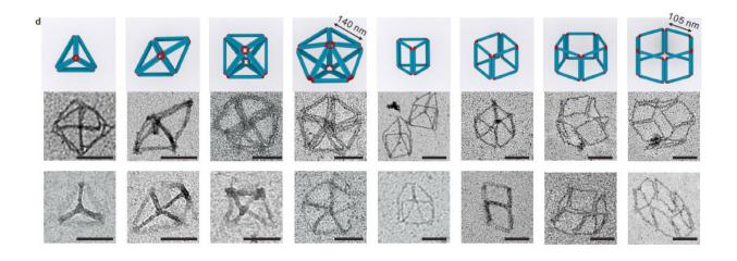
Models and transmission electron microscopy (TEM) images of various 3D polyhedra that were constructed by connecting the self-linked triangular M-DNA and rectangular M-DNA. From left to right: a tetrahedron, triangular bipyramid, octahedron, pentagonal bipyramid, triangular prism, rectangular prism, pentagonal and hexagonal prisms. Credit: Hao Yan
