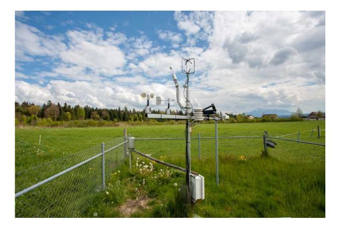
At the Chamau research station, these instruments measure the gas exchange between the ecosystem and the atmosphere with high frequency (20 Hz). Credit: ETH Zurich
