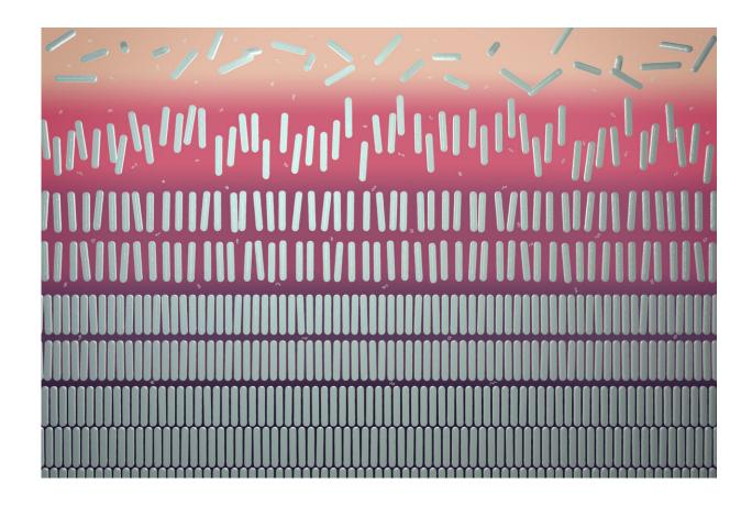
A five-phase equilibrium with at the top a gas phase with unaligned rods (isotropic phase), then a liquid phase with rods pointing in about the same direction (nematic liquid crystal), subsequently a liquid phase with rods lying in different layers (smectic liquid crystal), and two solid phases at the bottom. Credit: ICMS animation studio
