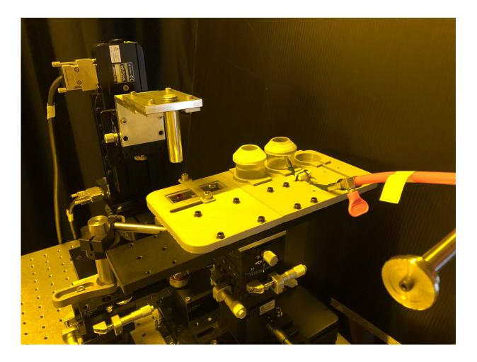
The researchers created a palette to hold multiple resins and placed it, two cleaning tanks and an air blow nozzle on a motorized stage. This allowed all the processes to be carried out sequentially for automated production of multicolor 3D microstructures. Credit: Shoji Maruo, Yokohama National University
