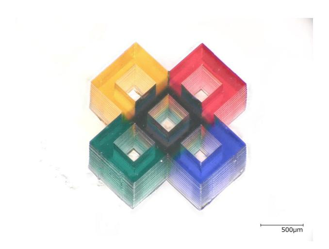
By adjusting the number of layers of multicolor resins, the researchers could adjust the light absorbance for each part of a structure. This allowed them to create black in microstructures such as this cross shape by combining layers of red, blue, green and yellow. Credit: Shoji Maruo, Yokohama National University
