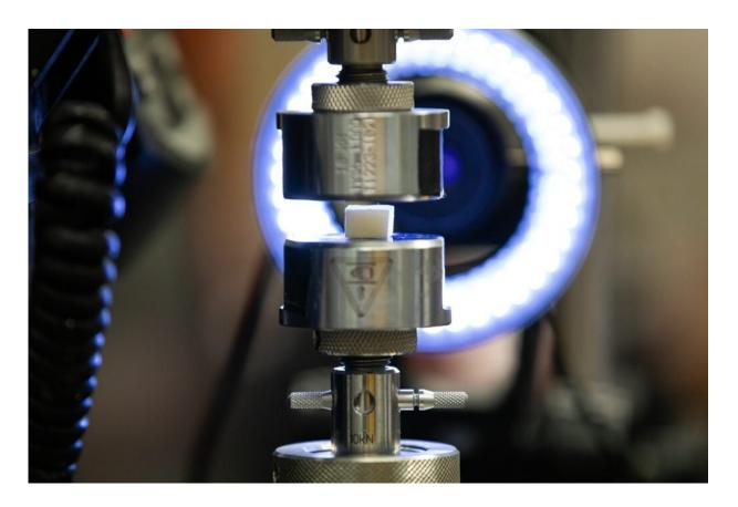
A cube-shaped sample isolated from cuttlebone is placed in a mechanical tester for compression measurements. Credit: Peter Means for Virginia Tech
