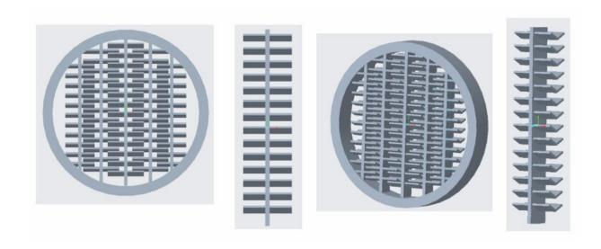
In the prototype of the mask's filter, a ring with V-shape "fins" was designed to increase the surface area where air passes through more channels. Credit: Jing Zhang, School of Engineering and Technology
