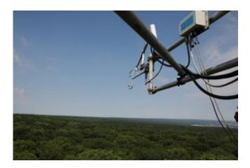
The carbon dioxide and water vapour exchange between forest and atmosphere has been continuously measured at the measuring tower every 30 minutes for 20 years. Credit: Alexander Knohl
