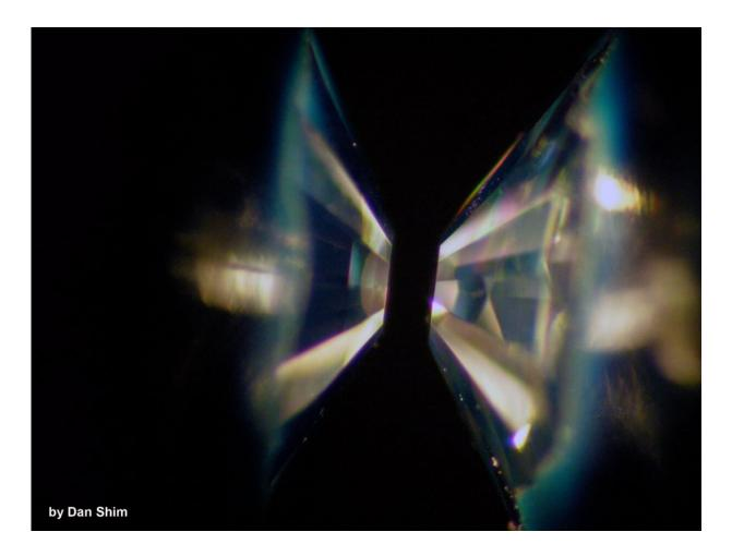
In a diamond-anvil cell, two gem quality single crystal diamonds are shaped into anvils (flat top in the photo) and then faced towards each other. Samples are loaded between the culets (flat surfaces), then the sample is compressed between the anvils. Credit: Shim/ASU
