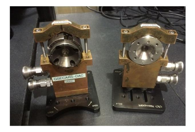
The cylinder-shaped objects in this photo are diamond anvil cells. The diamondanvil cells are mounted in copper holders and then inserted into the synchrotron X-ray/laser beam path. The photo shows diamond-anvil cells and mounts before they are aligned for X-ray/laser experiments. Credit: Shim/ASU
