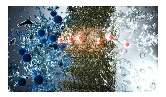
An artist's view of small-diameter carbon nanotubes that pass through water molecules (red and white) and reject ions (blue). High permselectivity of small-diameter nanotubes can enable advanced water desalination technologies. Credit: A. Noy, T. A. Pham, Y. Li, Z. Li, F. Aydin (LLNL). Illustration by Ella Maru Studios.
