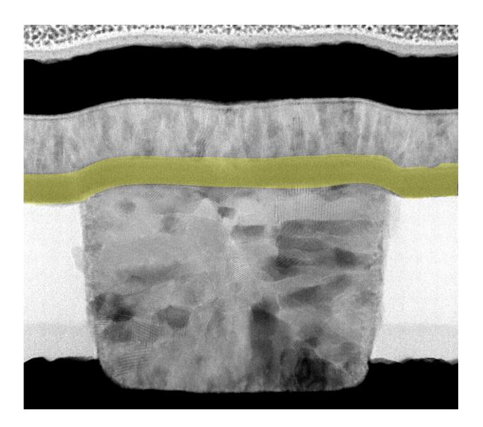
An electron micrograph of the artificial neuron. The niobium dioxide layer (yellow) endows the device with neuron-like behavior. Credit: Dr. R. Stanley
