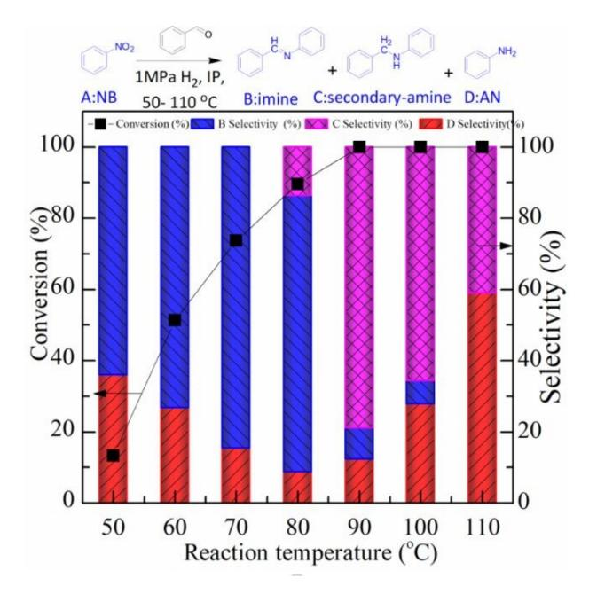
Figure 2. The catalytic activity of bi-metallic NiCo<sub>5</sub> catalyst in hydrogenation-coupling reaction. Credit: CHEN Chun
