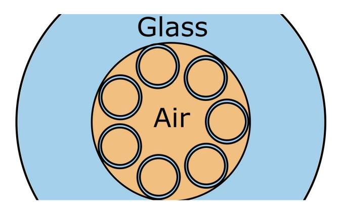
The anti-resonant hollow core fiber features a unique arrangement of seven hollow capillaries arranged around a hollow core inside the fiber. Credit: Arjun Iyer/Renninger lab/University of Rochester
