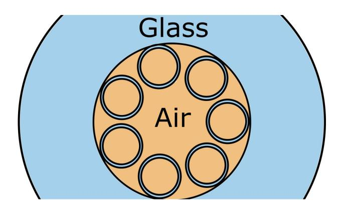
The anti-resonant hollow core fiber features a unique arrangement of seven hollow capillaries arranged around a hollow core inside the fiber. Credit: Arjun Iyer/Renninger lab/University of Rochester
