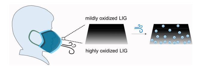
The team fabricates a hygroelectric generator to measure the change in the moisture-induced voltage when the user breathes through the graphene mask. Credit: *ACS Nano* (2020). DOI: 10.1021/acsnano.0c05330
