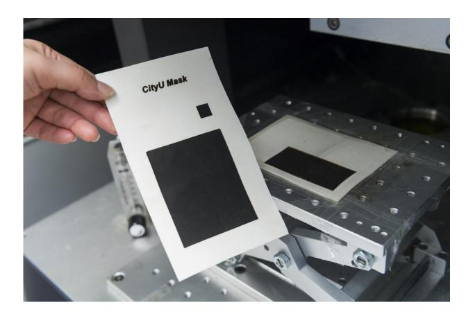
Most carbon-containing materials can be converted into graphene using a commercial CO2 infrared laser system. Credit: City University of Hong Kong
