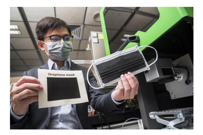
Dr Ye's team uses the  $CO_2$  infrared laser system to generate graphene. Experiment results show that the graphene they produced exhibit a much better anti-bacterial efficiency than activated carbon fibre and melt-blown fabrics. Credit: City University of Hong Kong
