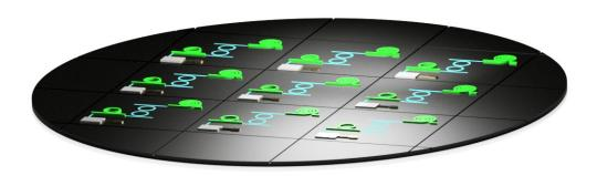
Wafer with both passive components of silicon nitride and the new amplifiers of erbium-doped aluminum oxide. Credit: University of Twente
