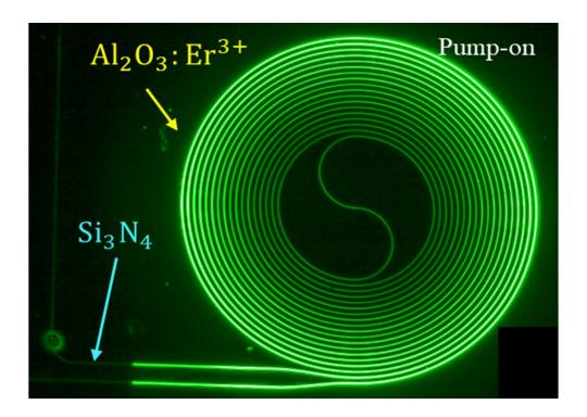
Optical amplifier setup with aluminum oxide and erbium. Credit: University of Twente
