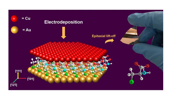
Copper thin films are created by electrodeposition of copper, Cu(111), on a selfassembled organic monolayer of the amino acid L-cysteine on gold, Au(111). Credit: Bin Luo
