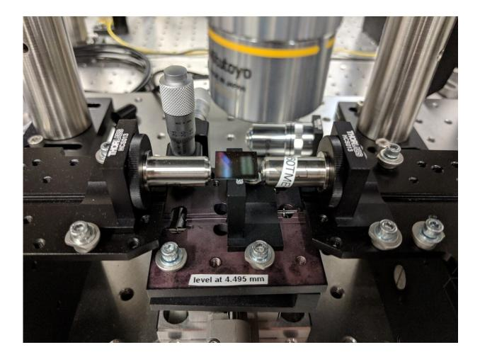
Chip-based nanophotonic nonlinear waveguides were a key component in this new system because they allowed very efficient conversion of light from one wavelength to another to create the supercontinuum. A close up of the nonlinear waveguide chip is shown here. Credit: David R. Carlson, National Institute of Standards and Technology and the University of Colorado in Boulder
