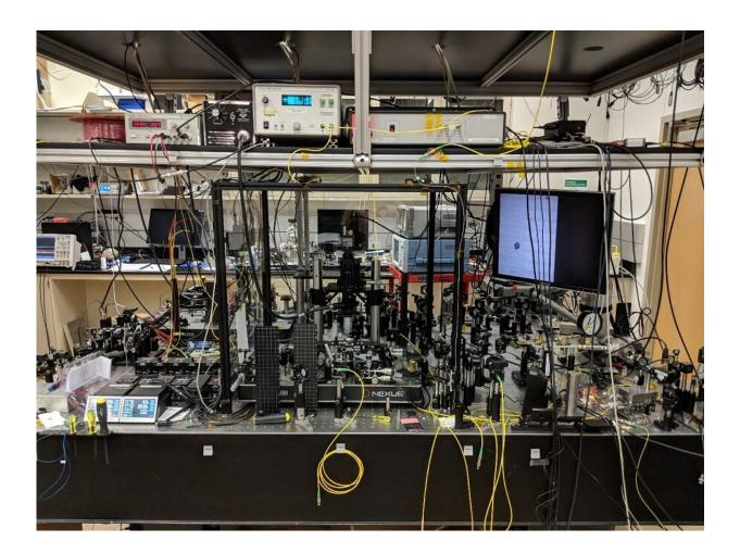
Researchers report the first dual-comb spectrometer with an acquisition speed of 10 gigahertz. The optical setup they used is shown here. Credit: David R. Carlson, National Institute of Standards and Technology and the University of Colorado in Boulder
