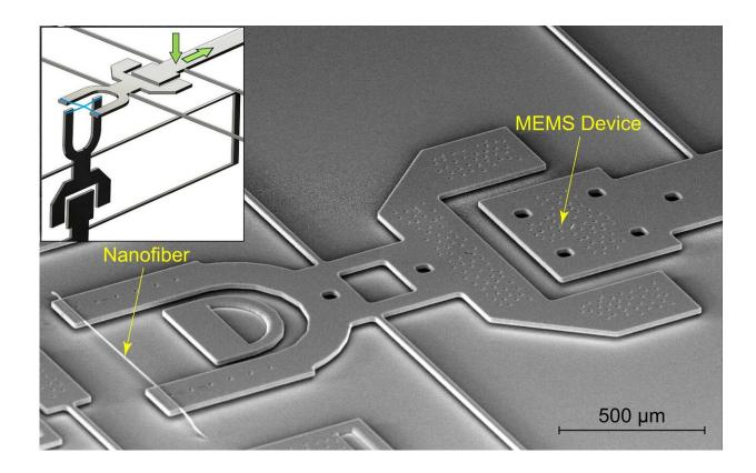
A polymer nanofiber, smaller than one hundredth the size of a human hair, mounted on a MEMS mechanical testing device. The inset shows two devices positioned perpendicularly so that adhesion and friction forces could be simultaneously measured at the intersecting point of contact. Credit: University of Illinois at Urbana-Champaign
