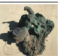
Water meter cover (green) that melted and fused to a meter and service line (brown/white/black)
