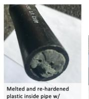
Pipes - melted plastic found within pipes
