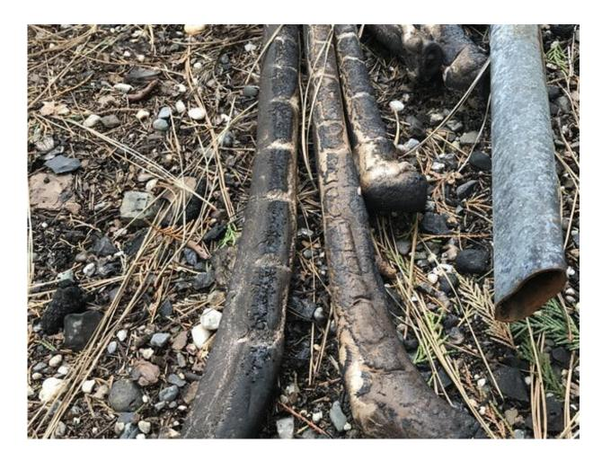
Plastic pipes can be damaged by heat and fire contact. Credit: Andrew Whelton, Purdue University
