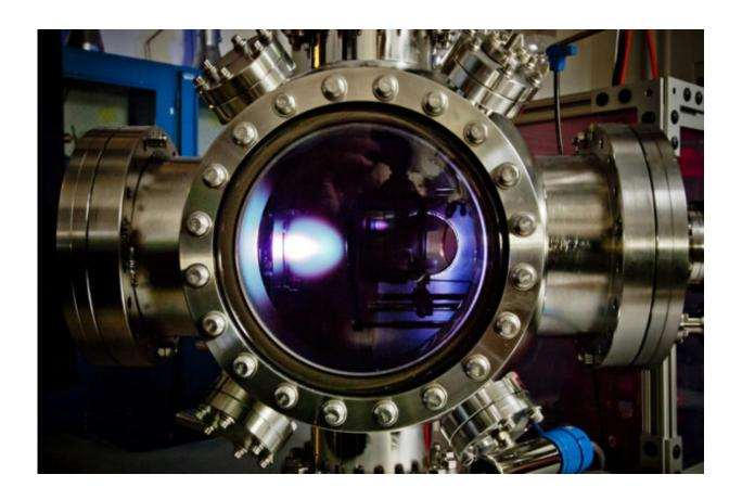
To make the new material, the thin film is first deposited via a pulsed-laser deposition process in this chamber. The bright "plume" you see is the laser hitting the target and depositing the material. Credit: Lane Martin.
