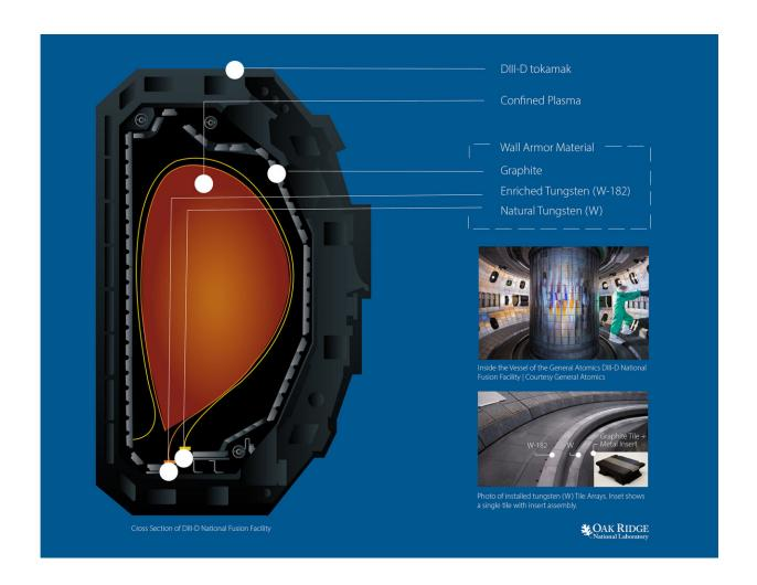
ORNL researchers used natural tungsten (yellow) and enriched tungsten (orange) to trace the erosion, transport and redeposition of tungsten. Tungsten is the leading option to armor the inside of a fusion device. Credit: Jaimee Janiga/ORNL
