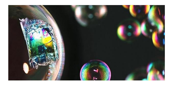
The fully printed ultrathin solar cell is light and flexible enough to rest on the surface of a soap bubble. Credit: 2020 KAUST; Anastasia Serin
