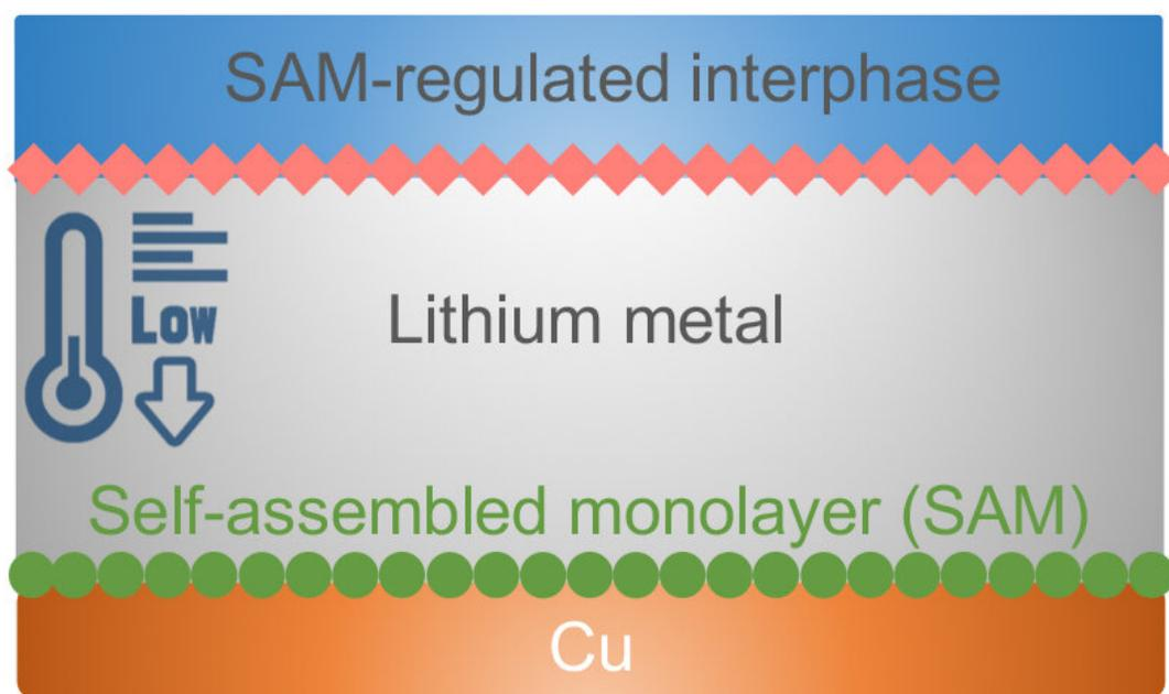
The layers in a lithium metal anode for low temperature batteries Credit: Donghai Wang, Penn State
