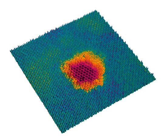
The projectile penetrates all layers, but only in the top layer, a big hole is created. The graphene below remains intact. Credit: TU Wien
