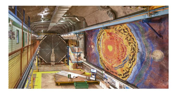
The MINOS+ and Daya Bay neutrino experiments have combined results to produce most stringent test yet for the existence of sterile neutrinos. In the MINOS+ experiment, Fermilab accelerators sent a beam of muon neutrinos through a detector located on the Fermilab site. The beam traveled 450 miles underground to a far detector, pictured here, in northern Minnesota. Credit: Reidar Hahn, Fermilab
