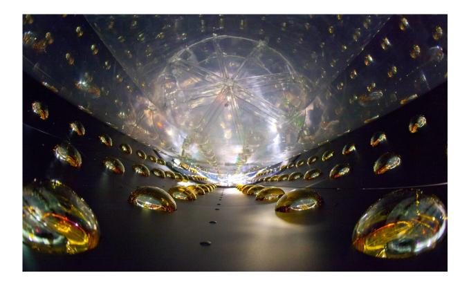
The Daya Bay neutrino detector walls are lined with photomultiplier tubes. The tubes are designed to amplify and record the faint flashes of light that signify an antineutrino interaction. Credit: Roy Kaltschmidt, Lawrence Berkeley National Laboratory
