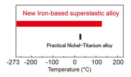
The temperature range of the new iron-based SEA compared to conventional metal-based SEAs for a stress change of 50 MPa. Credit: Tohoku University
