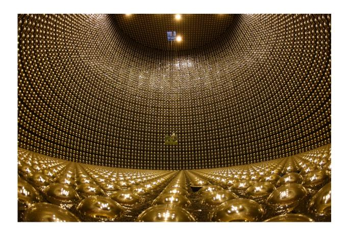
Inside Super-Kamiokande. The observatory is lined with 13,000 photomultiplier tubes which amplify weak flashes of light. Credit: Kamioka Observatory, ICRR (Institute for Cosmic Ray Research), The University of Tokyo
