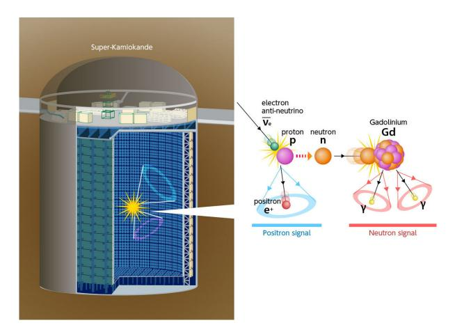
Neutrino interactions give off positrons and neutrons, neutrons strike gadolinium which then emits gamma rays. Credit: Kamioka Observatory, ICRR (Institute for Cosmic Ray Research), The University of Tokyo
