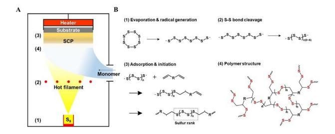
A schematic illustration showing the co-polymerization of vaporized sulfur to synthesize the high refractive index thin film. Credit: KAIST
