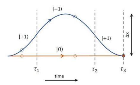
Space-time diagram of quantum states interference. By reversing the non-zero internal spin state at times \tau\_{1} and \tau\_{2} the particle can be made to follow the blue (spin +/-1) and orange (spin 0) paths. In doing so they reach a maximum spatial superposition size \Delta x before being brought back to interfere at time \tau\_{3} | Credit: R. Marshman et al
