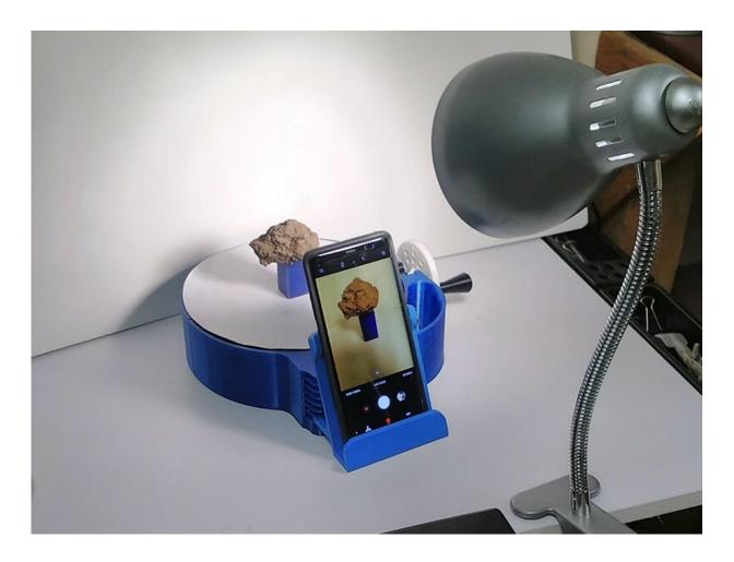
Experimental set up showing soil sample on a 3D-printed turntable with cell phone. A light provides consistent illumination while a white background and white turntable top reduce background influence. The soil sample is rotated on the turn table while taking an image every one fourth rotation. Credit: Colby Brungard
