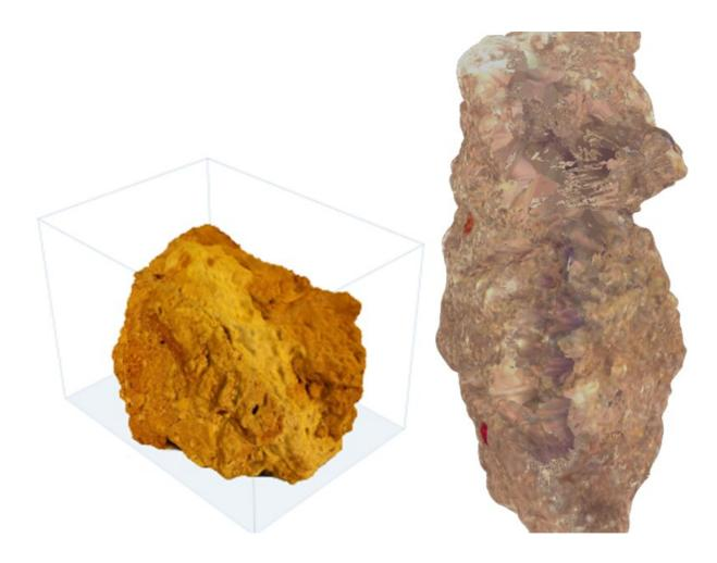
Examples of 3D renders derived from photogrammetry (left) and 3D laser scanning (right). The photogrammetry resulted in a render with the highest resolution. Credit: Colby Brungard
