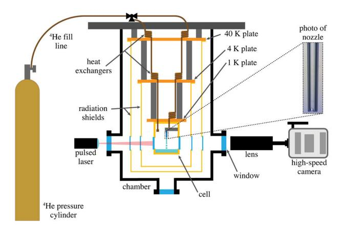
The experimental setup used by the team to capture the transformation of rapidly moving liquids into tiny droplets. Credit: KAUST
