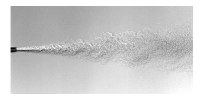
The team's high-speed camera images show how small surface perturbations and various forces cause a liquid tube to break apart into droplets. Credit: KAUST
