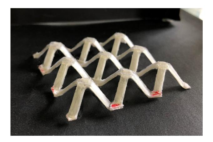
Combining silk fabric with epoxy creates laminates that can be formed into shapes, like the structure above, for medical uses. Credit: Jiao Wen & Juan Guan
