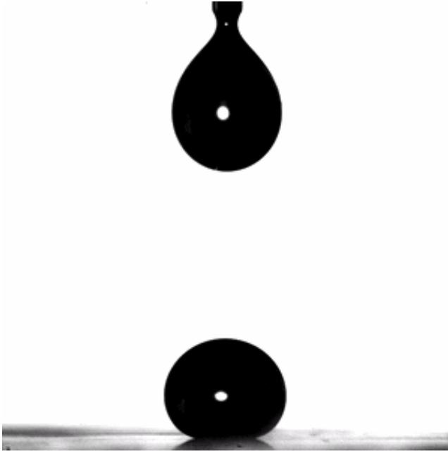
Experimental video of Case I for hexadecane drops: bouncing of impacting drop. (Weber number -
