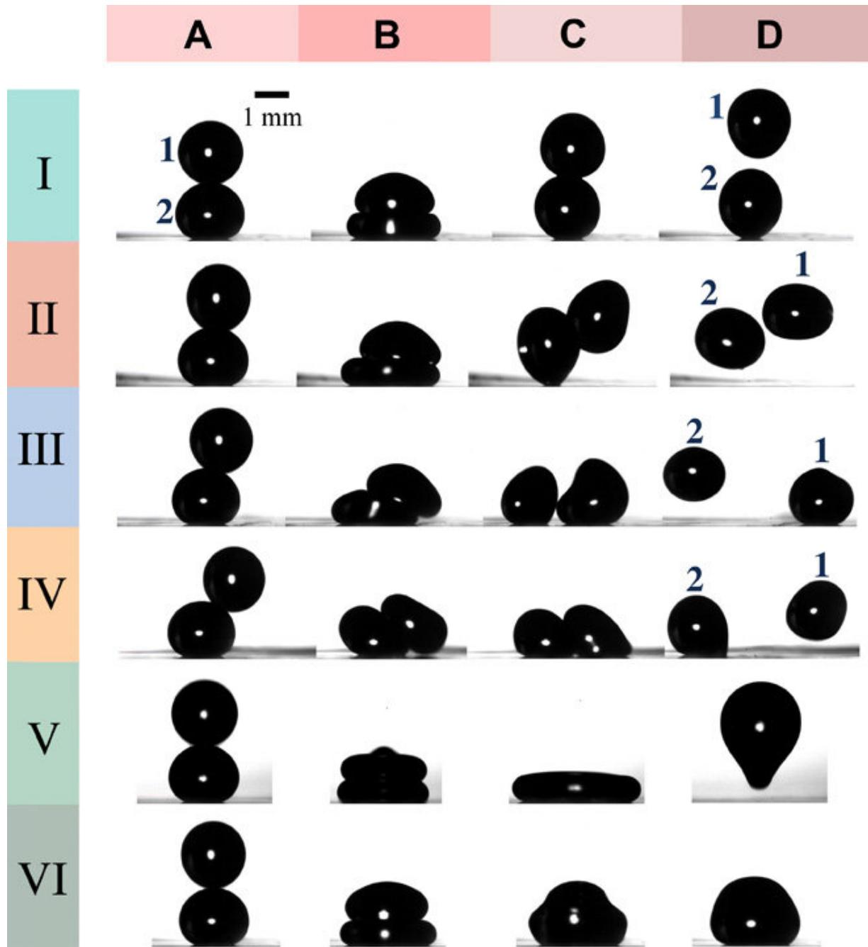
Snapshots of the impact dynamics. Note that the drop labels 1 and 2 are for the impacting and sessile drop, respectively. Six outcomes (cases I to VI) are observed when varying the impact parameter  $\chi$  and the Weber number ( $We$ ). The rows correspond to different impact parameter for I to IV. The columns show characteristic stages of the collision process. A, just at collision; B, sessile drop at maximum compression; C, droplet shape just before separation or
