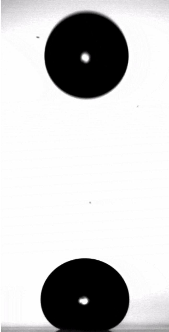
Experimental video of Case V (five) for hexadecane drops: coalescence of drops and lift-off of coalesced drop. Credit: Science Advances, doi:
