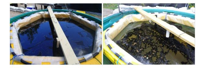
Comparison of the dilbit surface slick on Day 0 (left) and Day 8 (right). Left: The freshly added dilbit initially covers the water surface as a smooth slick. Right: Overtime the dilbit slick grew thicker, developed a surface crust and changed colour. Following heavy rain, roughly half the oil sank to the bottom. Credit: BOREAL Study 2017
