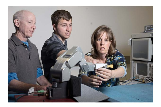
Rodney Leonhardt, Alec Weiss and Jeanne Quimby with NIST's SAMURAI, a portable measurement system to support design and repeatable laboratory testing of 5G wireless communications devices with unprecedented accuracy. Credit: Hammer/NIST
