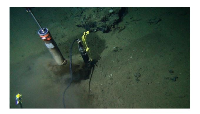
Photograph taken from ALVIN, a manned deep-ocean research submersible, taking sediment cores at the ocean floor of the Dorado Outcrop in 2014. Credit: Geoff Wheat, NSF OCE 1130146, and the National Deep Submergence Facility.
