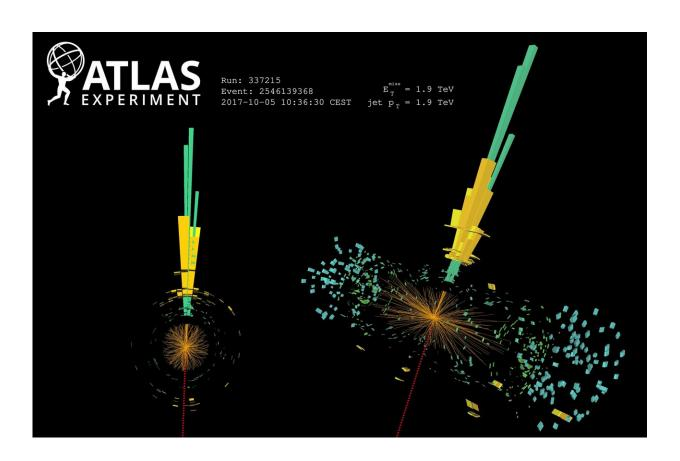
Figure 1: A monojet event recorded by the ATLAS experiment in 2017, with a single jet of 1.9 TeV transverse momentum recoiling against corresponding missing transverse momentum (MET). The green and yellow bars show the energy deposits in the electromagnetic and hadronic calorimeters, respectively. The MET is shown as the red dashed line on the opposite side of the detector. Credit: ATLAS Collaboration/CERN
