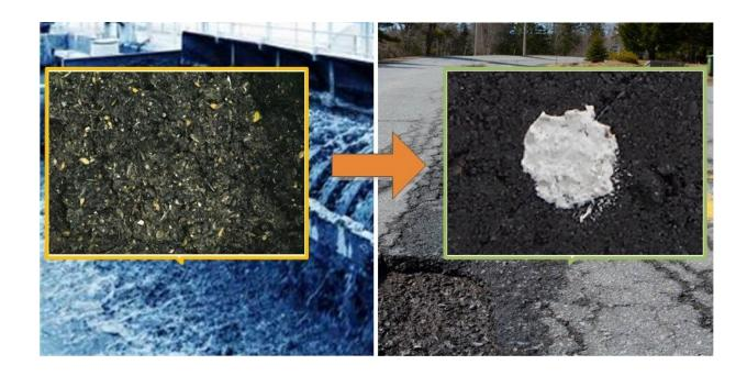
Researchers are turning grit from wastewater (left) into a ceramic mortar that can be used as pothole filler (right). Credit: Zhongzhe Liu
