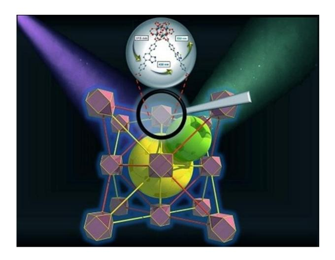
The metal-organic framework (MOF) contains zirconium-based nodes (lilac cuboctahedra) connected by carbon-based linker molecules (red and yellow rods) to form a porous structure with two large cavities (yellow and green spheres) in the crystalline material. The first linker absorbs ultraviolet light (315nm) and then transfers the energy as blue light (430 nm) to the second linker, which subsequently emits the energy as green light (530 nm). Credit: KAUST; Osama Shekhah
